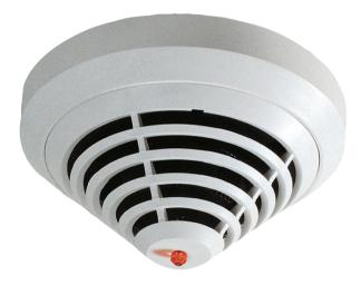
The FCP-320/FCH-320 Series Conventional Automatic Fire Detectors set new standards in fire detection technology through a combination of optical, thermal and chemical (gas) sensors and intelligent evaluation electronics. Their most impressive feature is their ability to prevent false alarms, as well as speed and accuracy of detection.
