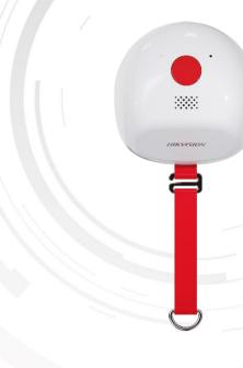
IRS-BVSMR3-H3AG is a millimeter-wave radar for vital sign monitoring based on the 60 GHz frequency band. The radar adopts the FMCW technology and comprehensively uses MIMO, beamforming, micro-Doppler feature extraction and other technologies to realize the detection of vital signs such as absence, respiration, heartbeat, etc.
